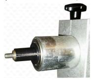
7) Fully insert the pulley, be sure to align one of the threaded hole of the pulley with the flat side of the adapter
