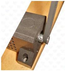
12) Preferably attach the motor to a surface that can be moved so you can further fine tune belt tension when system will be calibrated.
