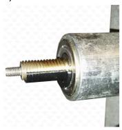
6) Put the second half, both parts need to be aligned and fully inserted in the thread
